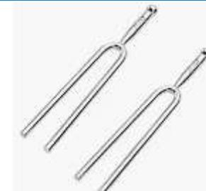
Tuning forks are made of metal. When you hit them on a surface, they vibrate and make a sound. The sounds are different pitches depending on the size and density of the fork you use. Some will make a higher pitched sound and some will make a lower pitched sound.
