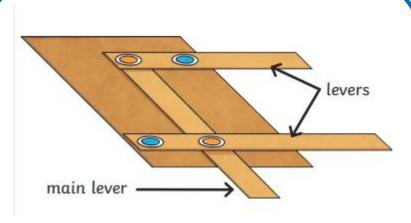
When the main level is moved, the linkages will move the two other levers.
